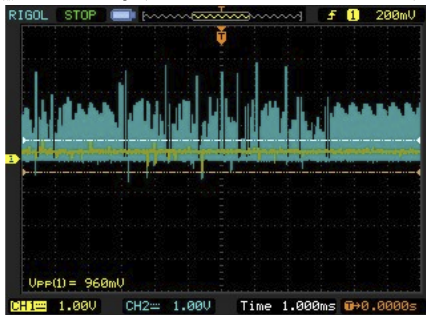
Figure 8: Signal I_{out} , Pre-filtered in blue, post-filtered in yellow
